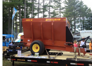
Mechanical Aerator and Wood Ash/Lime Spreader
